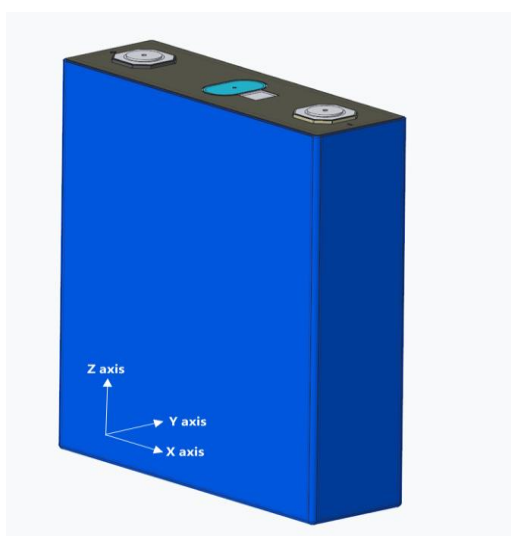
Fig.6 Diagram of LF230 Cell direction
